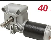
• Brand new, BUYERS PRODUCTS. High torque, right-angle gearmotor built to fit common truck and trailer tarp systems. Forged drive gear, aluminum gearbox housing and motor end-cap, steel motor housing. Gearbox is sealed to prevent contamination. Includes a chromed plastic bolt-on cover and mounting hardware. Shaft has two 5/16" cross-holes spaced 3/4" apart. Five mounting holes in face of gearbox tapped 5/16"-18.
